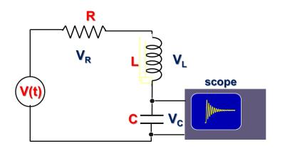
In this experiment R=300 ohms, C=1 $\mu$ F, L=33.43mH.
